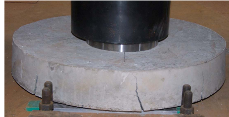
(b) The BFT and The initial crack development
