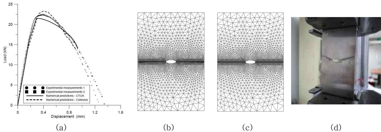
Fig 1. Horizontal crack: (a) Load–displacement curve; (b) Crack trajectory by CTOA; (c) Crack trajectory by cohesive model; (d) Experiment
